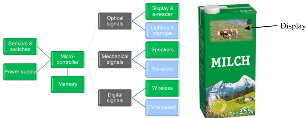
**Figure 6: Setup of a smart object: Milk package with integrated display, speaker, processor and power supply**
