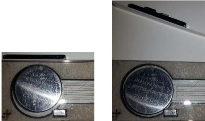
**Figure 12: Battery switch showing coin cell, two magnets and printed silver lines <sup>[6]</sup>.(Left: Box closed – switch off; right: Box open – switch on)**
