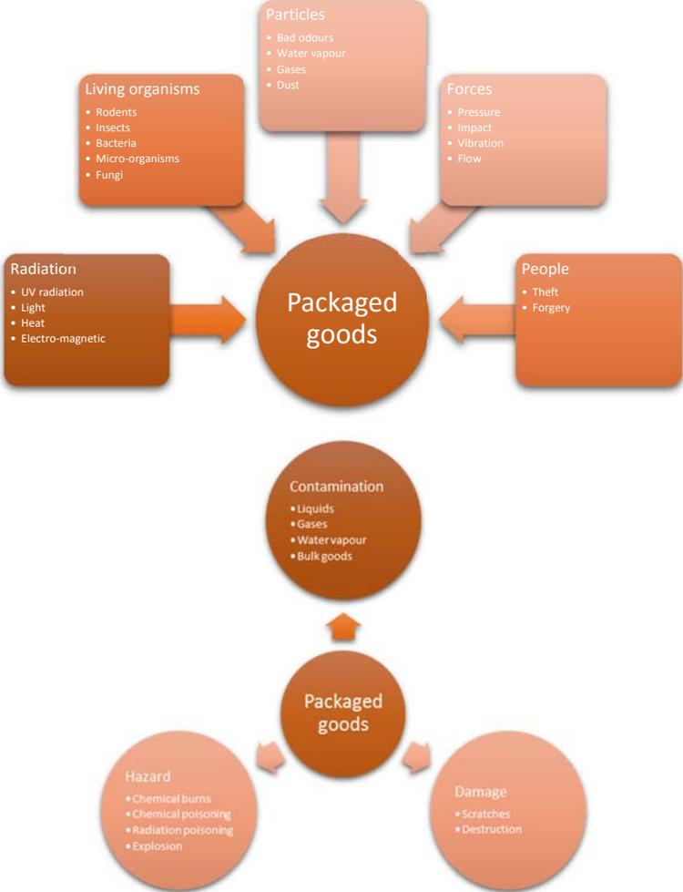
**Figure 1: Packaging function protection (top: protecting the packed goods against environmental impact; bottom: protecting the environmental against the packed goods)**
