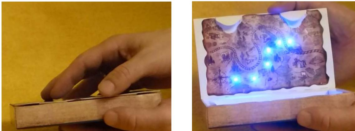
**Figure 13: Package with battery switch<sup>[6]</sup>.(Left: Box closed – switch off; right: Box open – switch on)**
