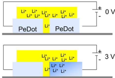
**Figure 9: Function of an electro-chromic display (Top off and bottom on)**
