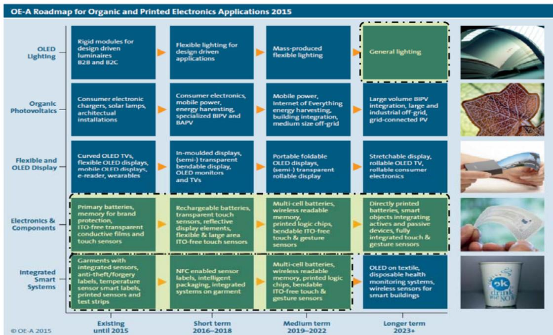
**Figure 4: OE-A Roadmap<sup>[4]</sup> for organic and printed electronics, with forecast for the market entry in large volumes (general availability) for different applications. Relevant areas for packaging are marked.**
